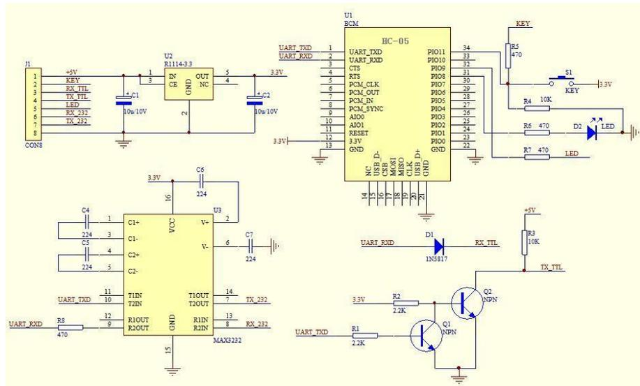
We provide two variations of BTM-5 breakout board, one is RS232 interface, the other is TTL interface. Note that these two different breakout board use different supply voltage and different interface, please take care before using them.
